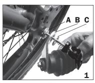
3. Insert the washer "C" on the quick-release skewer and slide the quick release into the axle.
